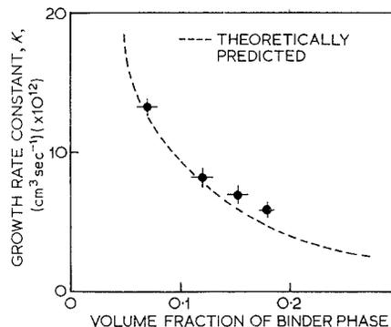
Figure 5 Effect of binder phase content on the grain growth of VC in VC-Co alloys; dotted line shows effect predicted by Equation 4.
