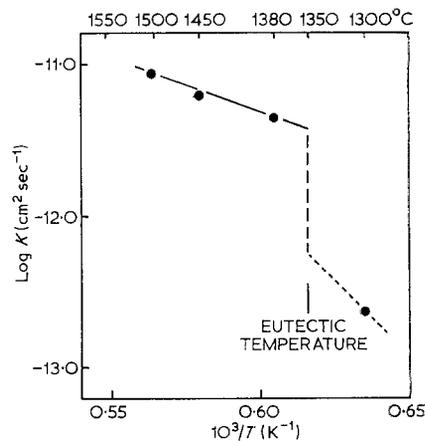
Figure 4 Effect of temperature on the grain growth of VC in the alloy VC-20 vol % Co.
