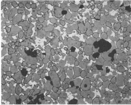
Figure 1 Microstructure of the alloy VC-20 vol % Co at the start of sintering;  $T = 1380^\circ\text{C}$ ,  $t = 0\text{ min}$  ( $\times 280$ ).
