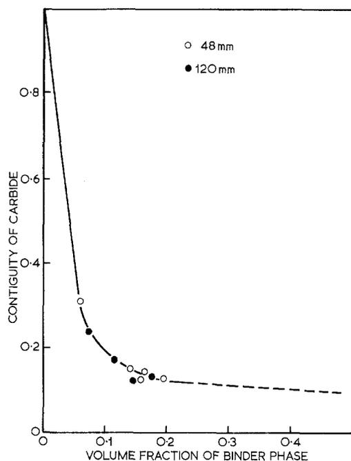
Figure 6 Effect of binder phase content on the contiguity,  $G(t \geq 48 \text{ min}; T = 1450^\circ\text{C})$ , of the VC grains in VC-Co alloys.
