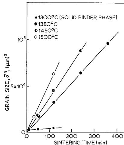
Figure 3 Grain growth of VC in the alloy VC-20 vol % Co, plotted as  $\bar{d}^3$  versus  $t$ .
