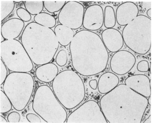
Figure 2 Microstructure of the alloy VC-20 vol % Co sintered at  $1380^\circ\text{C}$  for 120 min ( $\times 280$ ).
